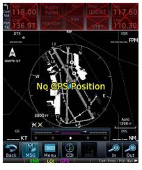
If data fields become invalid, the GTN typically annunciates the failures with a large red X, as shown.
